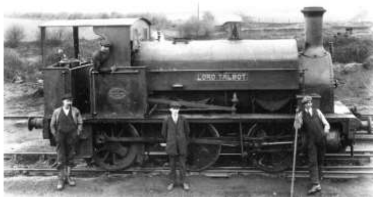
The colliery loco Lord Talbot employed for shunting and conveying trucks to/from Parkgate, built by Black, Hawthorn & Co, Gateshead, 1881
