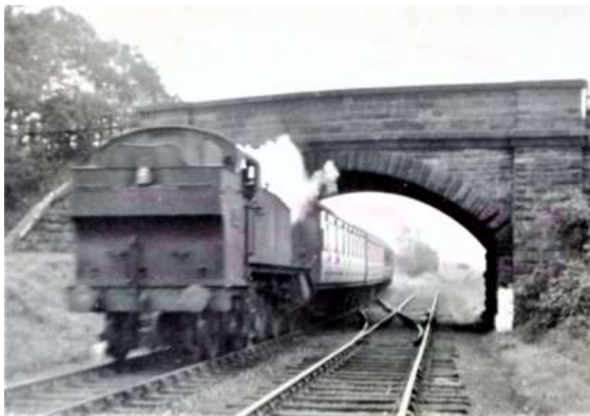
A short train for West Kirby makes its way down the grade from Neston towards Parkgate, bunker first. The location is Moorside Lane bridge, where the freight line from Neston Colliery (right-hand track) joins the line from Hooton. The loco is one of Birkenhead's ex-GWR 4575 class small prairie (2-6-2) tank engines.
